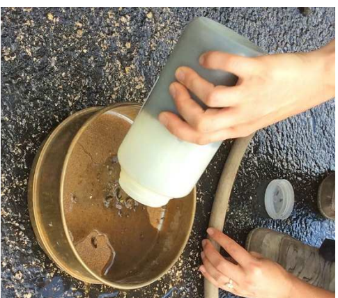
Sediment samples were poured into a mesh sieve in order to filter out small particles
