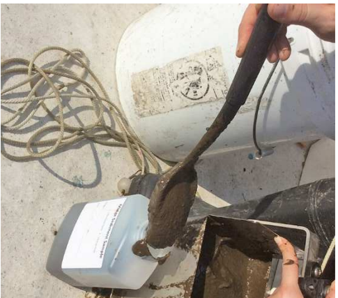
Sediment samples were transferred into a Nalgene bottle in order to transport sediment samples to Aquatic Systems, where larval counting took place
